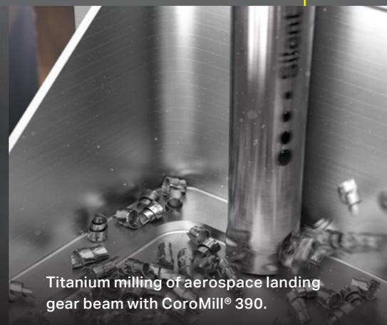
Titanium milling of aerospace landing gear beam with CoroMill® 390.
