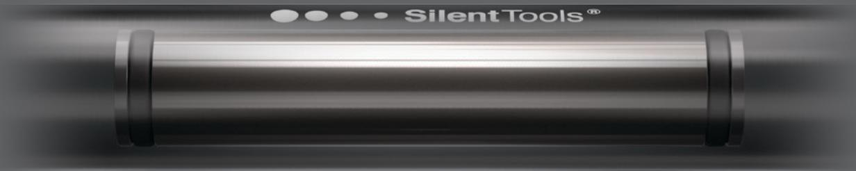
Inside the tool is a pre-tuned damping system that consists of a heavy mass, supported by rubber spring elements. If vibration arise, the kinetic energy will be absorbed by the damping system. This leads to minimized vibration and greatly improved productivity.
